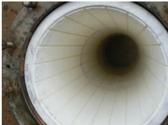
Figure 4. Bushing coated with Thordon SXL
