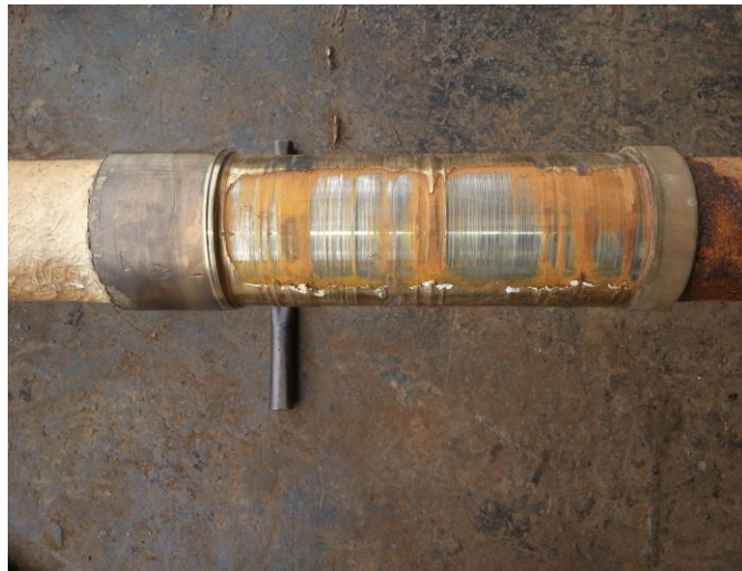
Figure 5. Bronze sleeve wear
