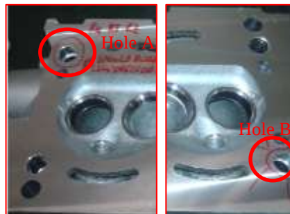
Fig. 4 – Holes A and B generated by the 12.150 mm drill.
