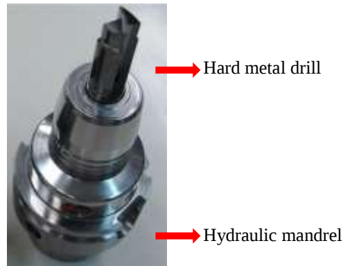
Fig. 3. – Housing of the hard metal end steel VK5drills
