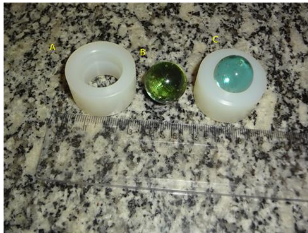
Figure 1. Mould the Van Gogh membranes shows A) support, B) glass mould and C) coupling to generate the latex lamina using this technique.
