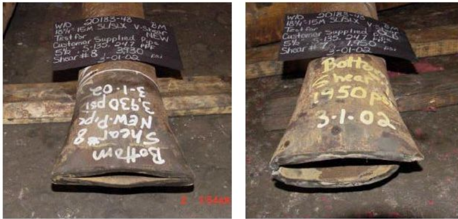
Figure 4. Two pipes after the BOP cutting process (Childs et al. , 2004).
