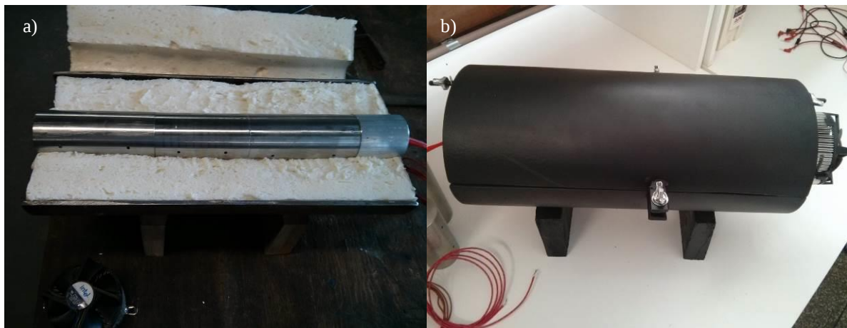
Figure 11 – Thermal conductivity meter apparatus assembly a) Opened apparatus. b) Closed apparatus.
