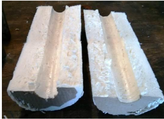
Figure 6 – Thermal insulator constructed of polyurethane.
