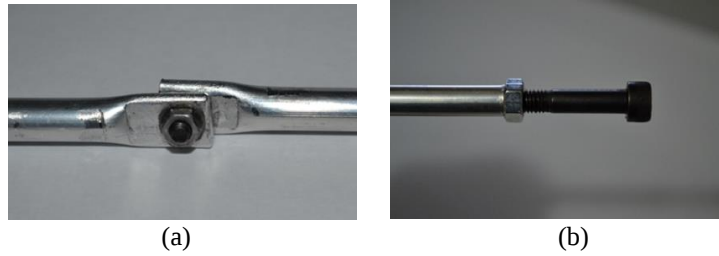
Figure 3. (a) Photo of the manufactured flat joint; (b) Bolt used in the linking of bar elements in perpendicular planes.
