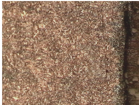
Figure 2. Workpiece's raw material micro-structure (100% martensitic)
