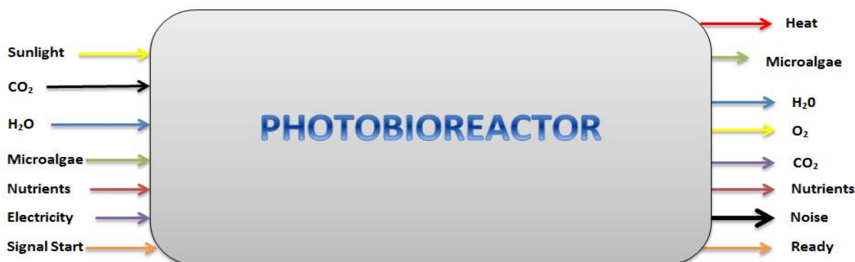
Figure 2. Function Structure Diagram (FSD) by the Black Box Method
