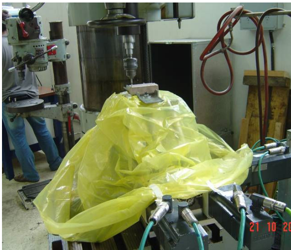
Figure 9. (a) Parallel mechanism at transverse machining plane (b) Work piece after parallel traverse machining
