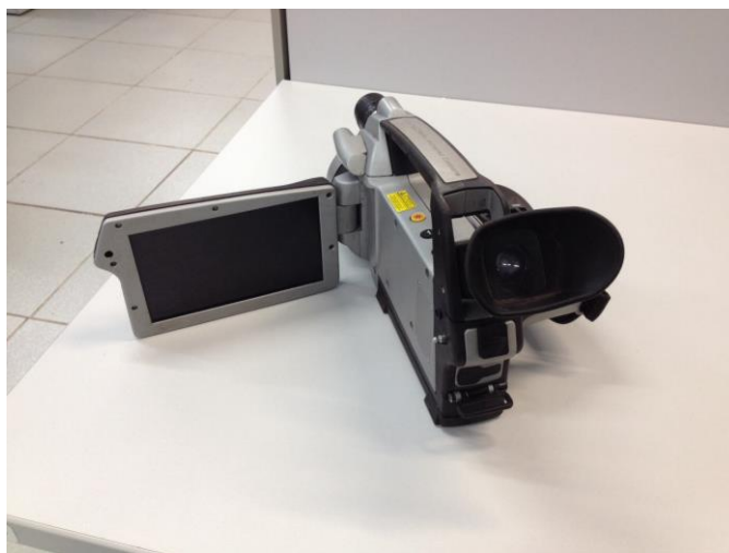
Figure 3. Thermographic Camera utilized: FLIR P640
