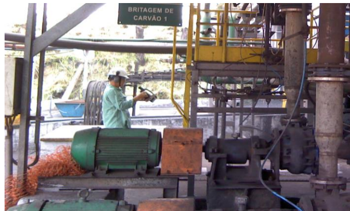
Figure 5. Inspector using the Thermographic Camera
