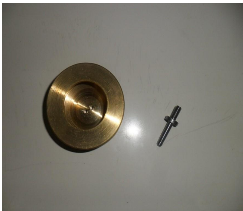
Figure 2. Disk and pin used in the tests in pin-on-dink equipment.
