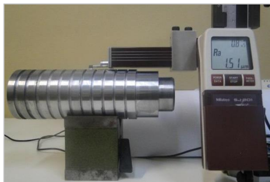
Figure 7. Surftest SJ-201P used in the roughness surface measurement.
