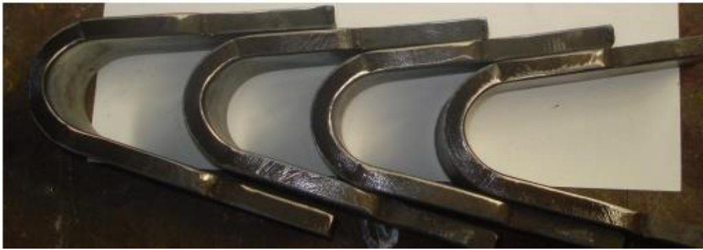
Figure 8. Detail of samples after bending tests
