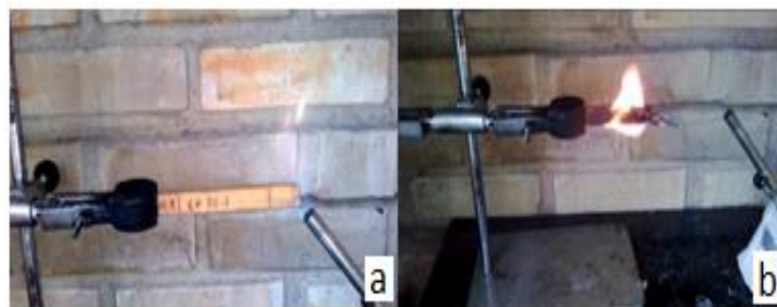
Figure 14. UL-94 HB test the CP-35 composite: (a) Flame application for 30 seconds; (b) Sample completely burned
