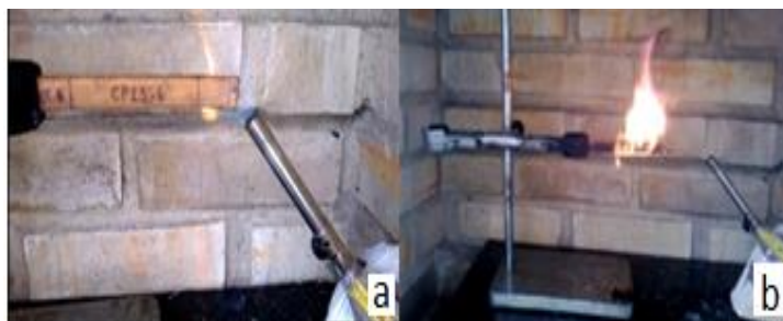
Figure 12. UL-94 HB test the CP-15 composite: (a) Flame application for 30 seconds; (b) Sample completely burned
