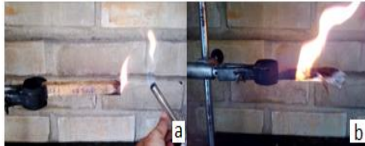
Figure 13. UL-94 HB test the CP-25 composite: (a) Flame application for 30 seconds; (b) Sample completely burned
