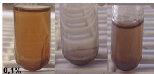
Figure 2. Copper oxide nanoparticles dispersed in toluene, hexane and ethylene glycol, respectively.
