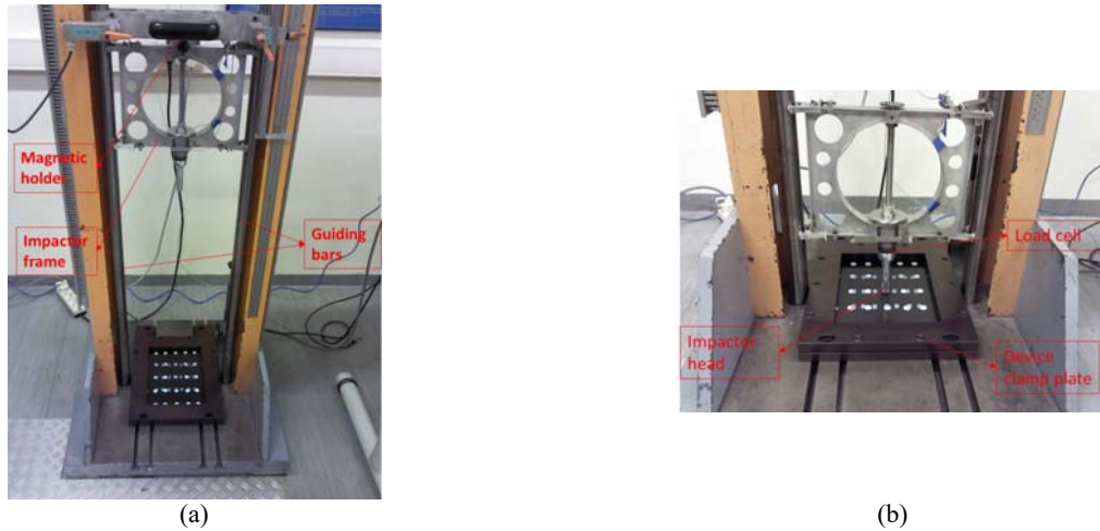
Figure 1. (a) Experimental set-up of the impact test and (b) test specimen on the basis of the drop tower
