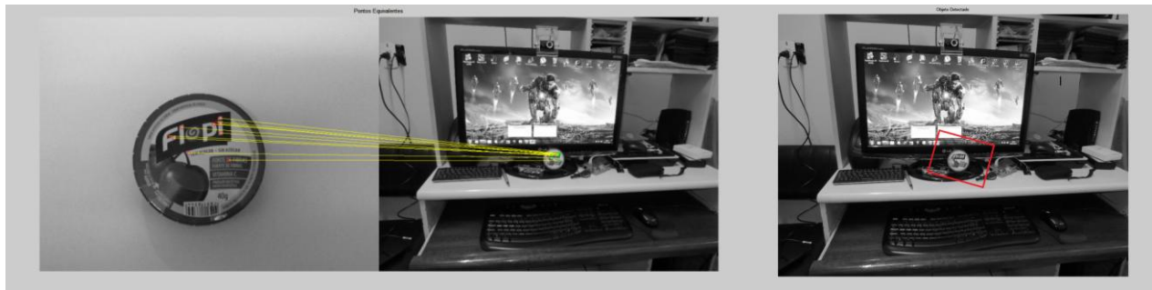
Figure 11 – Identification of equivalent characteristic points of a complex object using SURF algorithm.
