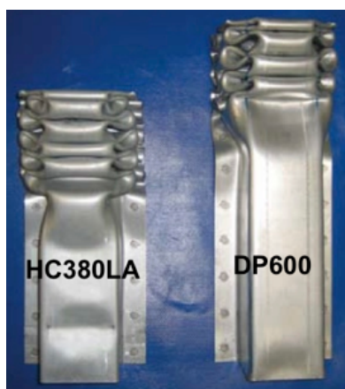
Figure 7. Comparison of deformation of HC380LA and DP600 steels. (Corus, 2009)
