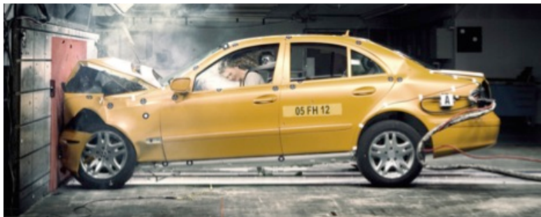
Figure 6. Frontal crash test. (WorldAutoSteel, 2009)
