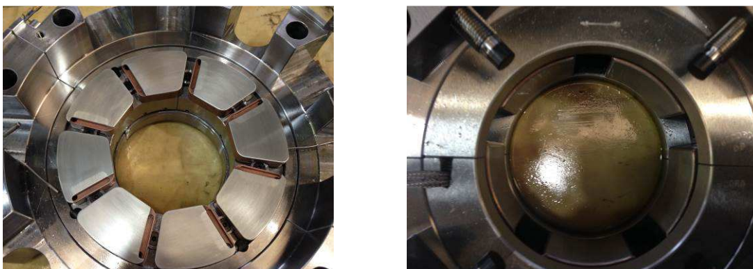
Fig. 2. Left: Thrust bearing. Right: Journal bearing
