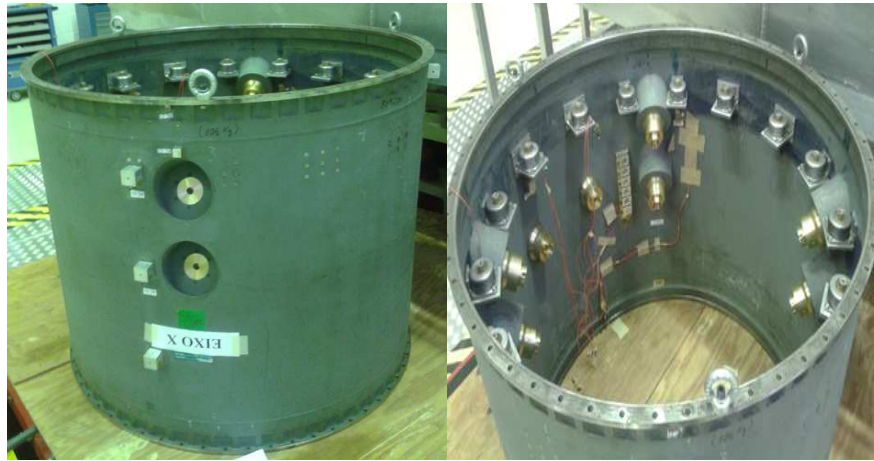
Figure 2. Satellite Launch Vehicle (VLS) equipment bay structure
