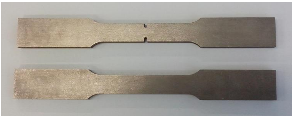
Fig. 2. Specimens used in tensile tests
