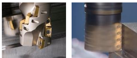
Figure 1 – Tangential milling cutter contact and the machined surface
