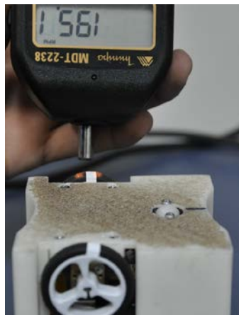
Figure 4. Measure of RPM of wheel with tachometer, showing value of 195,1 RPM.
