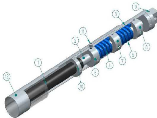
Figure 1. HSEA's components: (1) hydraulic cylinder; (2) movable rod; (3) base tube; (4) and (5) springs; (6), (7) and (8) guides; (9) load terminal; (10) connection guide; (11) guide bolt; (12) encapsulation tube.
