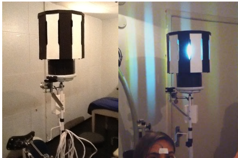
Figure 5. Assembly used in the evaluation of the device for stimulation of optokinetic nystagmus.
