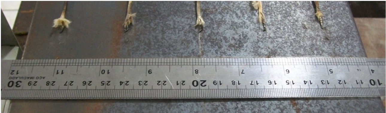
Figure 2. Thermocouples position along the center of the sheet.
