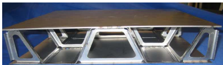
Figure 2. Thermally Integrated Structural Sandwich Core (TISSC) – NASA concept.
