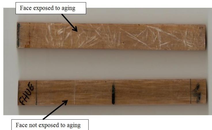
Figure 3. Comparison between the two faces after the accelerated environmental aging test.
