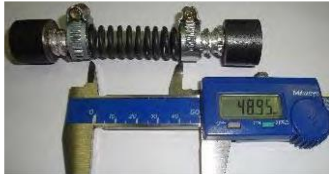
Figure 1. Spring of SMA Ni-Ti
