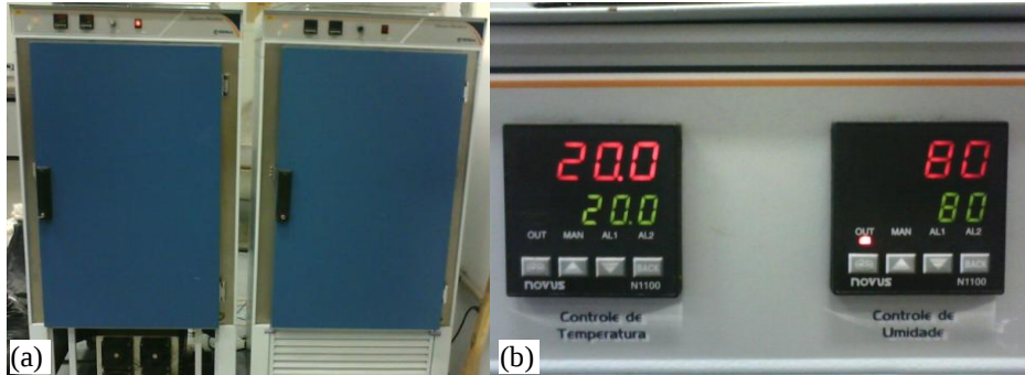
Figure 2. (a) Automatic climate control used in obtaining the moisture classes; (b) Automatic climate control Display indicating the temperature and relative humidity, respectively.
