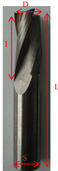
Figure 4. Tungsten carbide cutter with helical cuts to finish. Identification of their basic dimensions (D, L, I e S)
