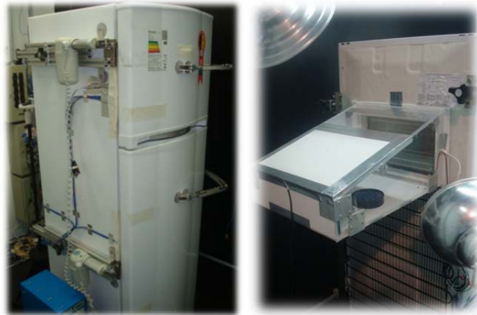
Figure 7. Door-opening device (left) and visualization improvement (right).
