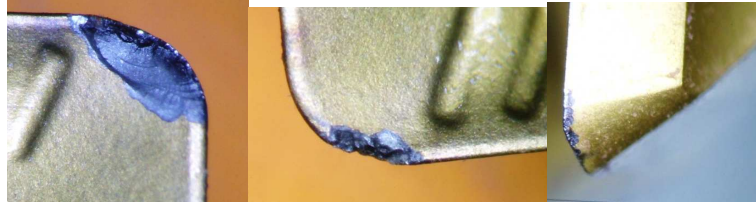
Figure 2 – Crater wear and flank wear on the insert with 2 cutting edges with conventional lubrication
