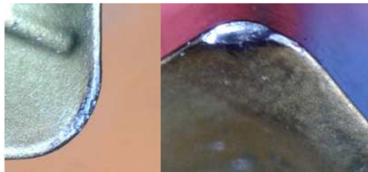
Figure 3 –Flank wear on the insert with 2 cutting edges for the frontal milling using MQF and a chipping on the insert with 4 cutting edges for the frontal milling using MQF
