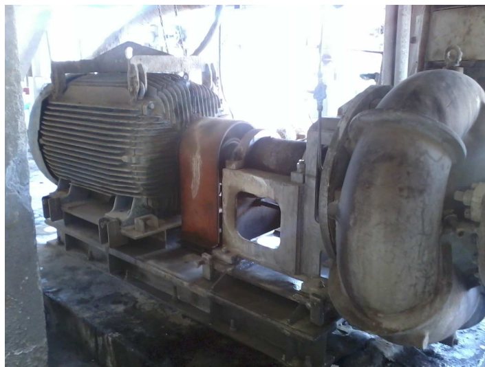
Figure 3. Image of the centrifugal pump case used in the analysis of the cavitation.
