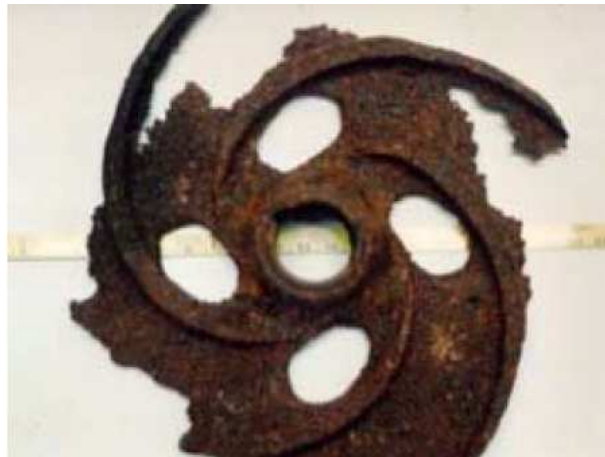
Figure 1. Damage of the centrifugal pump rotor caused by the cavitation.
