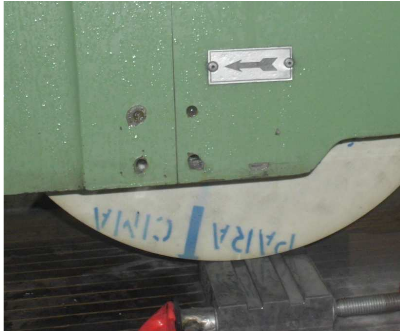
Figure 3. Flat grinding test of ABNT 4340 quenched and tempered steel.
