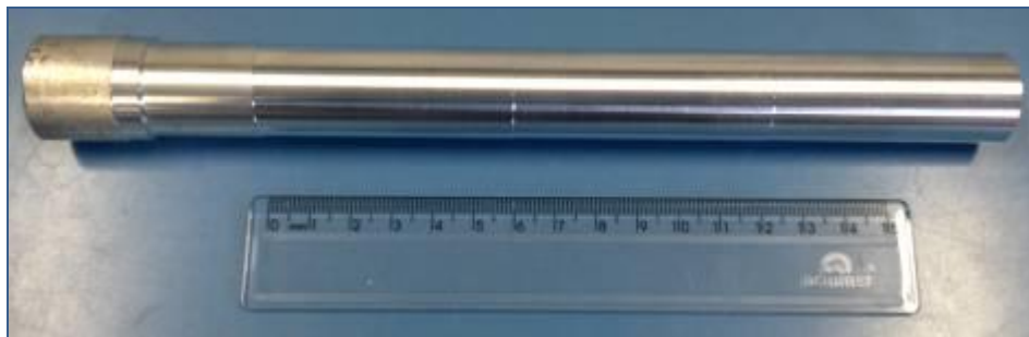
Figure 2 – Aluminum Alloy 2024 tested sample.
