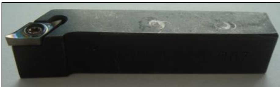
Figure 6 – Carbide tool coated with TiB_2 .
