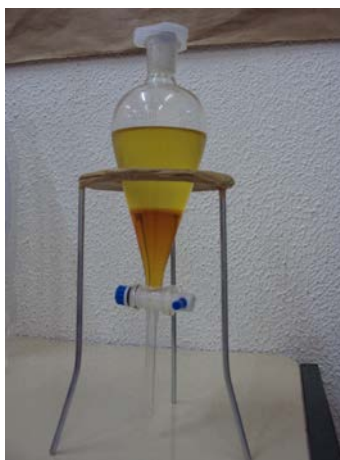
Figure1. Biodiesel top phase and glycerin bottom phase (Carlos, 2014).
