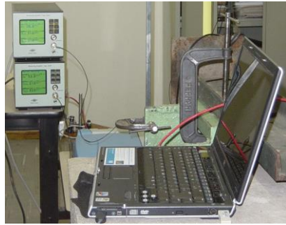
(a) Amplifiers and portable computer
