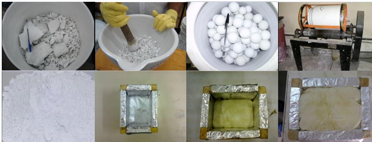
Figure 1. Process fabrication steps of the specimens
