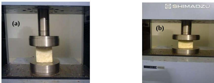
Figure 2. Application of (a) preload and (b) compressive load in the specimen
