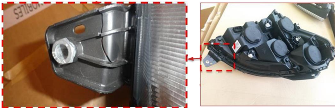
Figure 2. Head Lamp critical anchorage and most common reported failure
