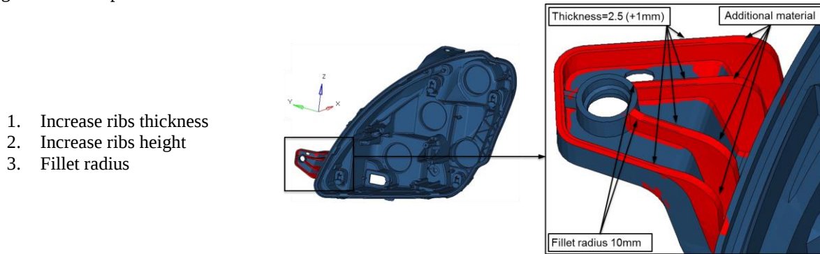
Figure 7. Proposed modifications at original head lamp
