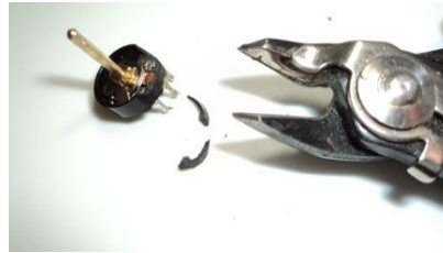
Figure 8 - Withdrawal latch potentiometer (FerPinheiro page in WordPress, 2014)
