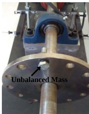
Figure 12a. Unbalanced Mass in the perforated disc.
