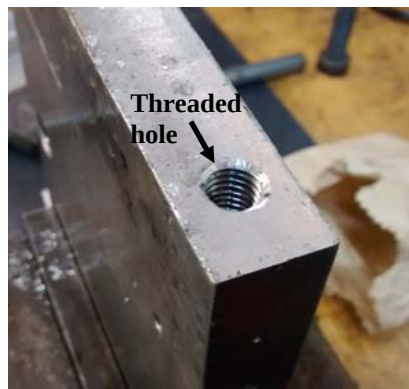
Figure 7b. Threaded hole in detail.
