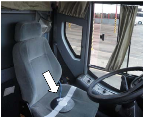
Figure 1(a). Location of the seat pad accelerometer at the seat/operator interface
