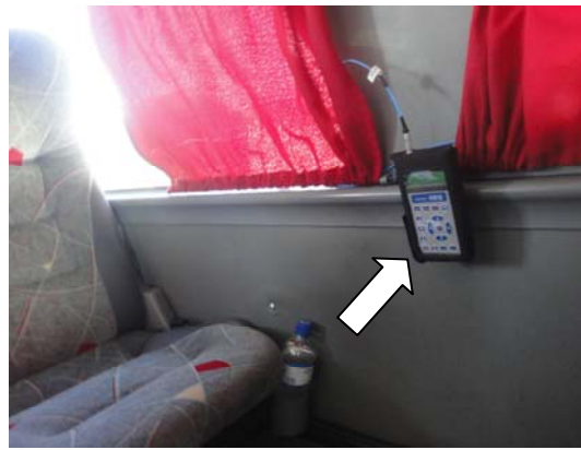
Figure 1(b). Location of the handheld vibration analyzer at the bus (behind the driver seat).
