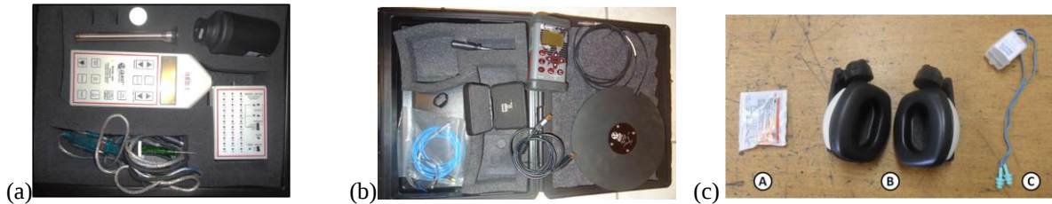
Figure 3. (a) Sound pressure level meter Quest 1900 model. (b) Vibration level meter Quest VI-400Pro (c) Hearing protection, (c-a) moldable earplug, (c-b) protective earplug shell, (c-c) protective precast earplug.
