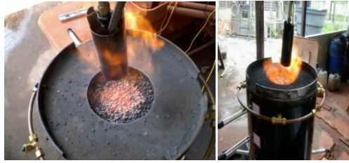
Figure 3- Combustion Ignition of the solid fuel in the combustion cell
