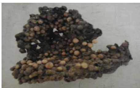
Figure 5. Aspect of pellets after sintering process during the combustion reaction.
