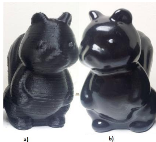
Figure 2 –Example of object before(a) and after(b) smoothing process
