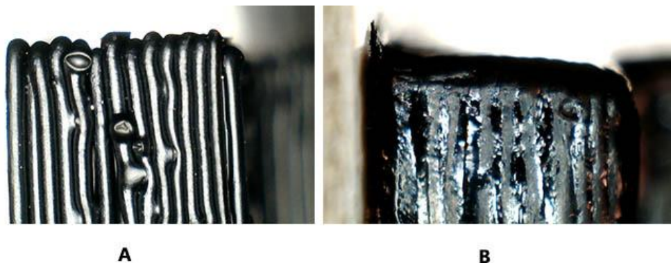
Figure 10 – Comparison between object surface at before smoothing process (A) and after 16th pass (B)
