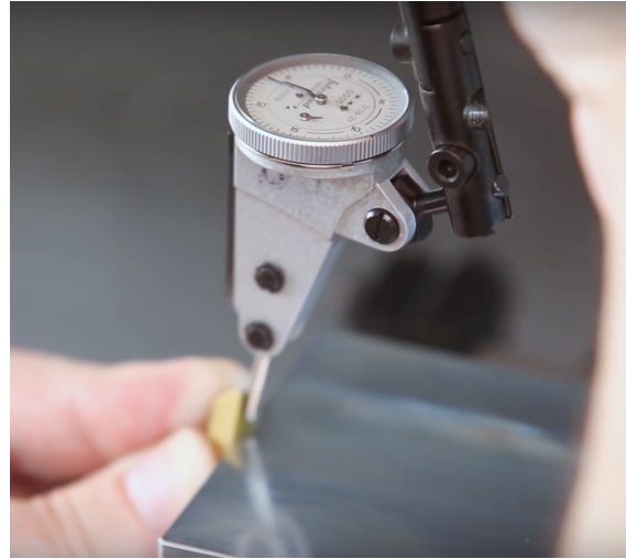
Figure 11: Finding y-axis with an indicator (b)
