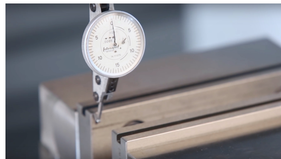
Figure 9: Indicator touching-off the vise
