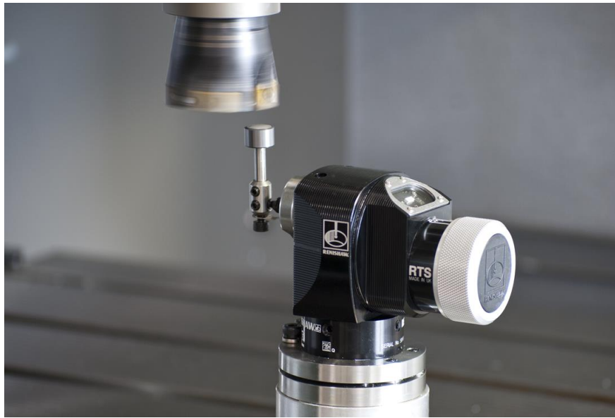
Figure 7: Tool probe mounted in a vertical machining center
