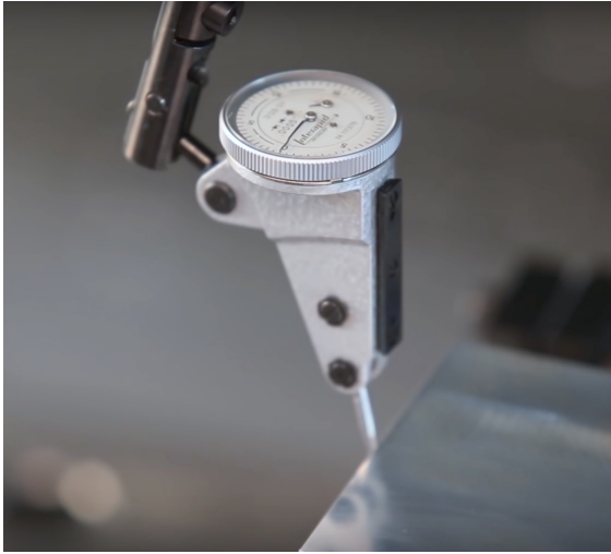
Figure 10: Finding y-axis with an indicator (a)
