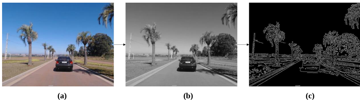
Figure 8. (a) An acquired RGB image is converted to (b) grayscale image and (c) the edges are detected using canny filter.
