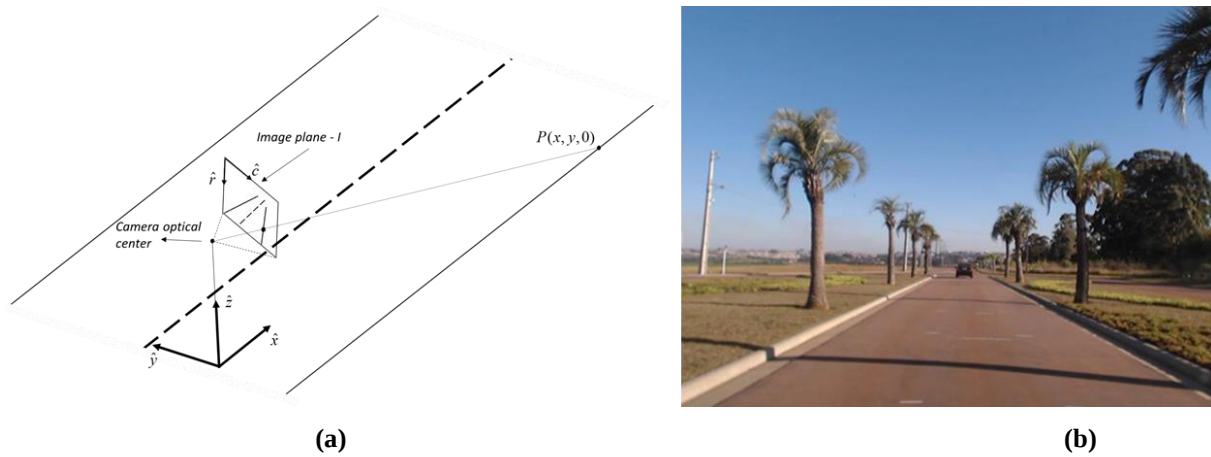
Figure 1. (a) Projection of a point P from the 3D world on the image plane I and (b) The perspective effect, note that the width of the highway changes according to the distance.
