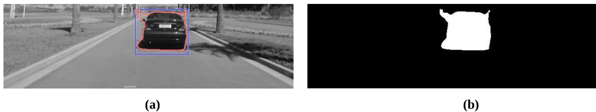
Figure 10. Active contour model applied to detect a vehicle: (a) in blue initialization curve and in red the detected vehicle edge and (b) the area corresponding to the vehicle.
