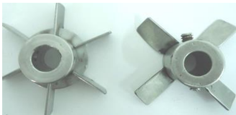
Figure 1. Rushton turbine to the left and oblique blade impeller to the right
