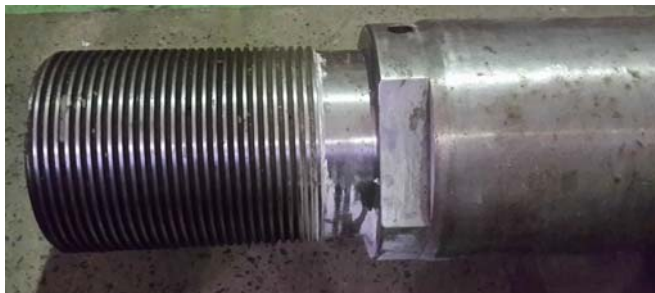
Figure 8. Threaded End of the Piston Rod
