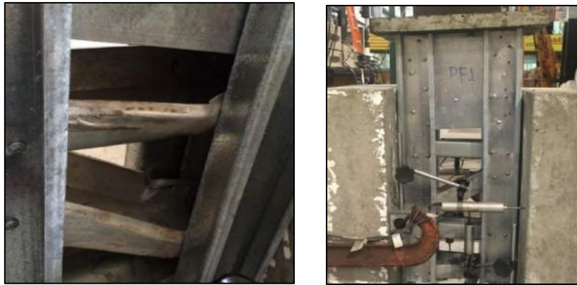
Figure 21 – Visible rotations associated with diagonals, vertical and top of the prototype
