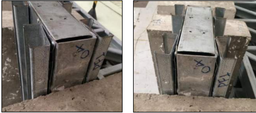
Figure 20 – Deformed configuration of specimen PF-1
